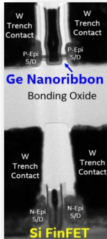
Sequential Approach W. Rachmady, IEDM, 2019
